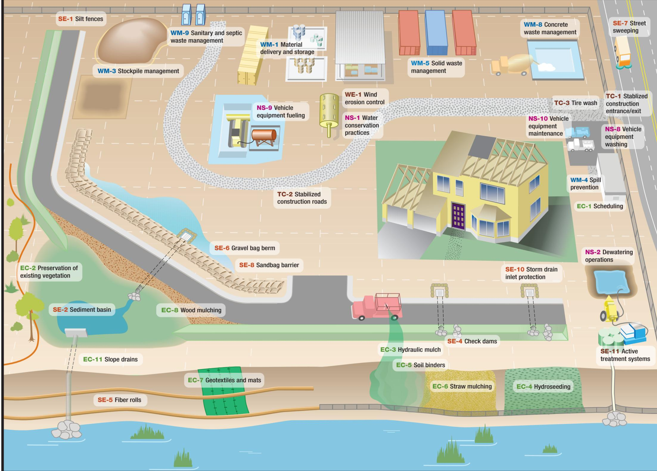
Stormwater runoff in the County drains directly into local creeks and into the ocean. Implementing Best Management Practices (BMPs) to keep construction site runoff clean is an important part of the County's program. This brochure describes BMPs that must be implemented for high risk construction projects within the County.
