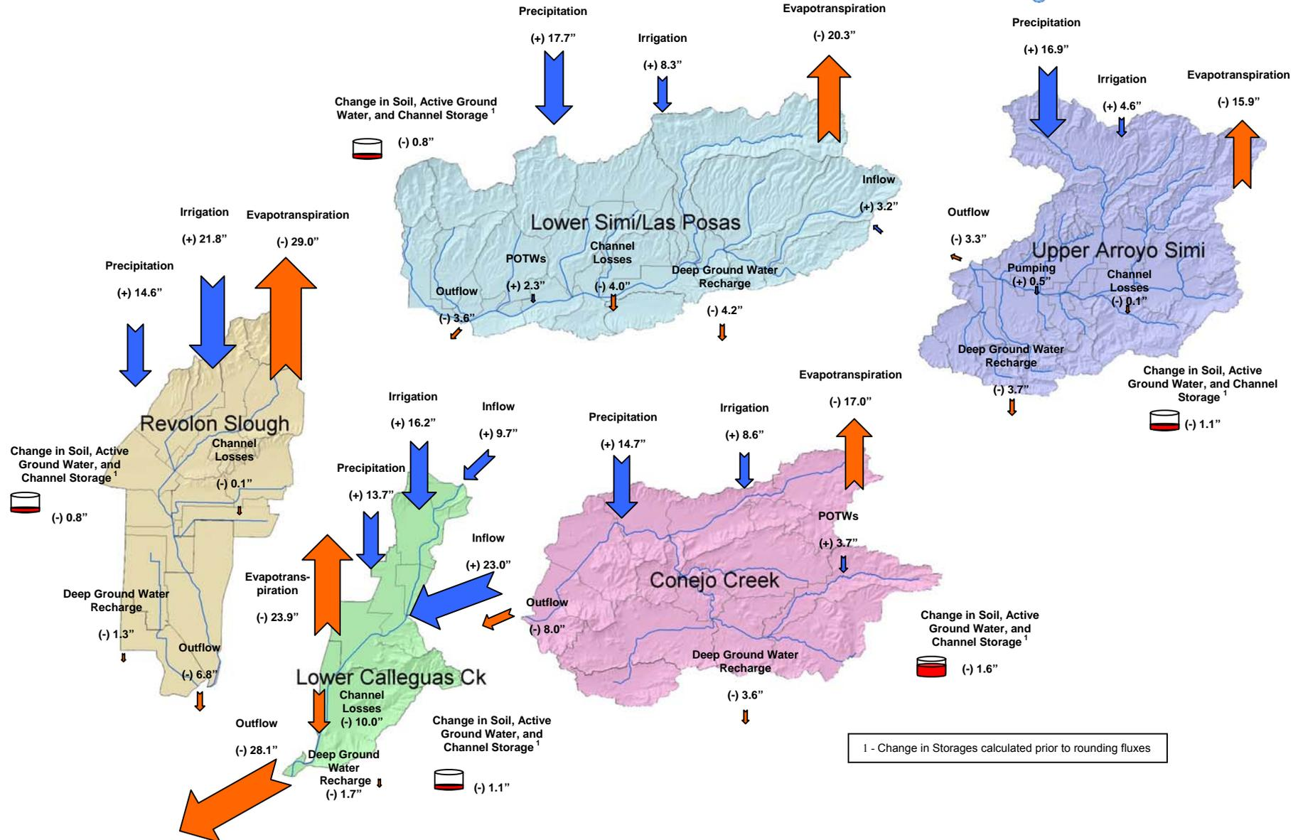
Figure 4.12 Water Balance Components for Subwatersheds of the Calleguas Creek Watershed for WT 1960 – WT 2002
