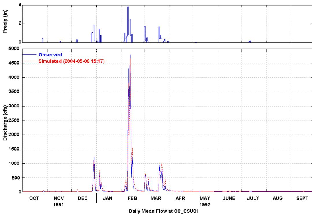
**Figure 4.5 Daily Flow Simulation at Calleguas Creek CSUCI for 1998 (Calibration) and 1992 (Validation)**
