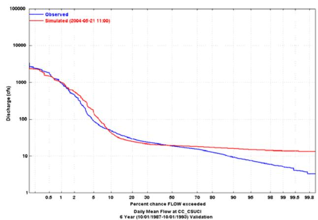
Figure 4.6 Calibration and Validation Flow Duration Curves at Madera, Conejo, and Calleguas Creek at CSUCI
