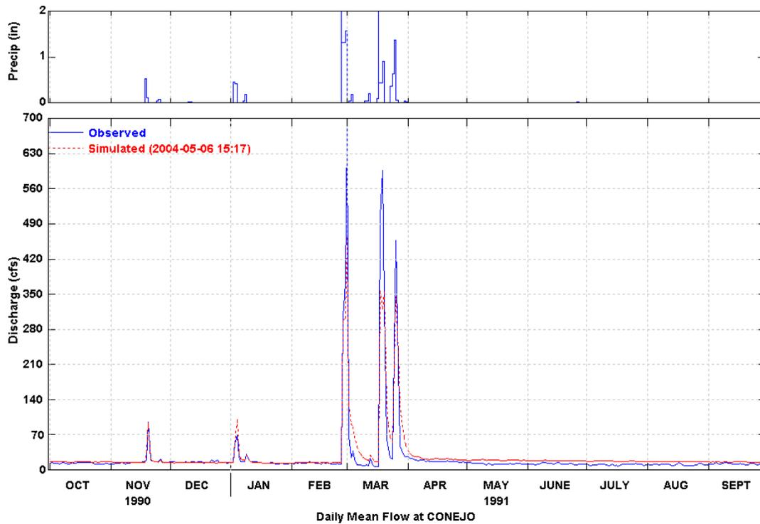
Figure 4.4 Daily Flow Simulation at Conejo for 1998 (Calibration) and 1992 (Validation)
