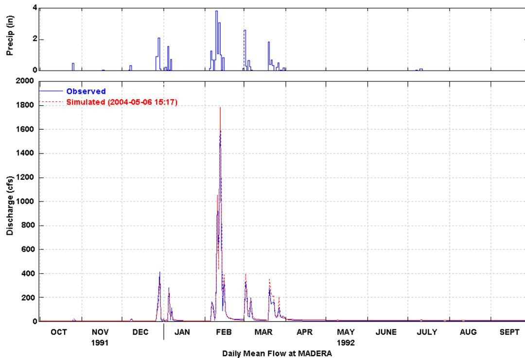
Figure 4.3 Daily Flow Simulation at Madera for 1998 (Calibration) and 1992 (Validation)
