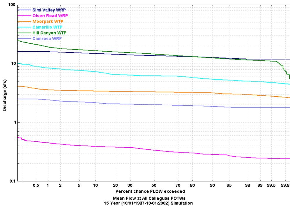
Figure 2.4 Flow Duration Curves for Calleguas Point Sources
