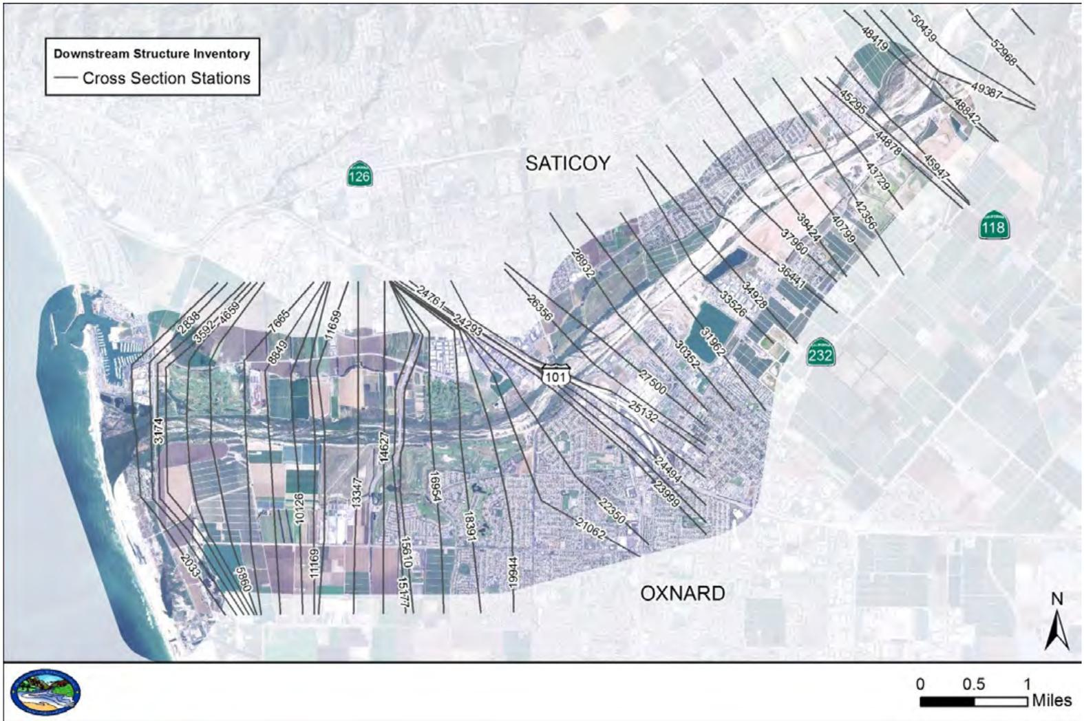
**Figure 8 – Cross Section Stations Used in HEC-FDA Model**
